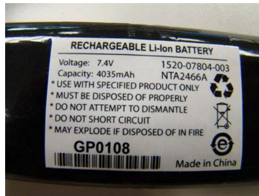
Battery Pack Date Code Example: GP0108 (January 2008) Battery Pack Part Number Example: 1520-07804-003
